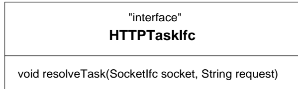
Figure A.7: Interface HTTPTaskIfc
