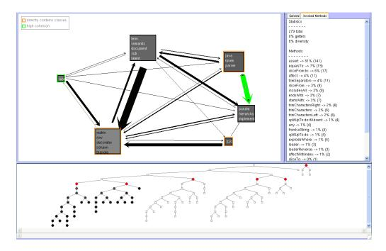
Figure 7.2: Hapax and Softwarenaut. On the left: the semantic clusters as boxes with arrows illustrating the number of invocations between them. On the right: the labels for the selected cluster. On the bottom: the dendrogram, a tree view of the clustering.
