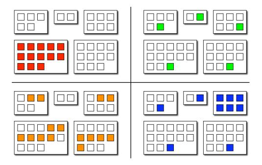
Figure 5.2: From top left to bottom right: a well-encapsulated concept that corresponds to the modularization, a cross-cutting concept, a design smell scattered across the system without much purpose, and finally an octopus concept which touches all modules.
