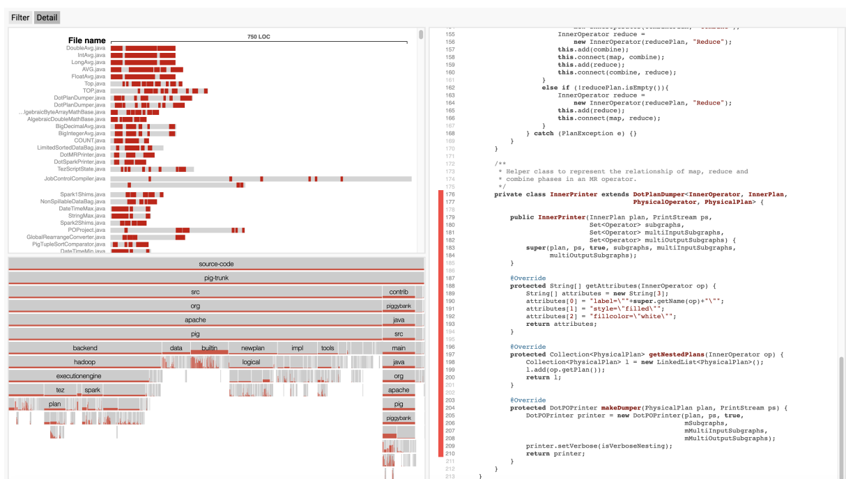
Figure 5.2: The detail tab of our tool shows the file graph (upper left), hierarchy graph (lower left) and the code view (right). The codebase being analyzed in the picture is apache pig. Checked out at commit 59ec4a326079c9f937a052194405415b1e3a2b06 at https://github.com/apache/pig/commits/trunk
