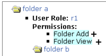
Figure 4.3: Setup to illustrate inheritance of roles. Wiki tree with two folders a and b . The role r1 is attached on folder a with permissions Folder Add and Folder View .
