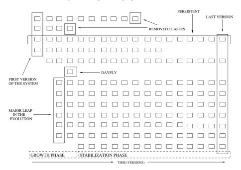
Figure 2. System level evolution aspects using the Evolution Matrix
