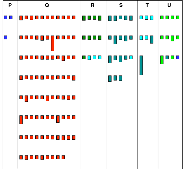
Figure 5. SYSTEM I Example. More than one color in a package indicates potential lack of locality. Size of smaller rectangles represent forces pulling the class towards the package.
