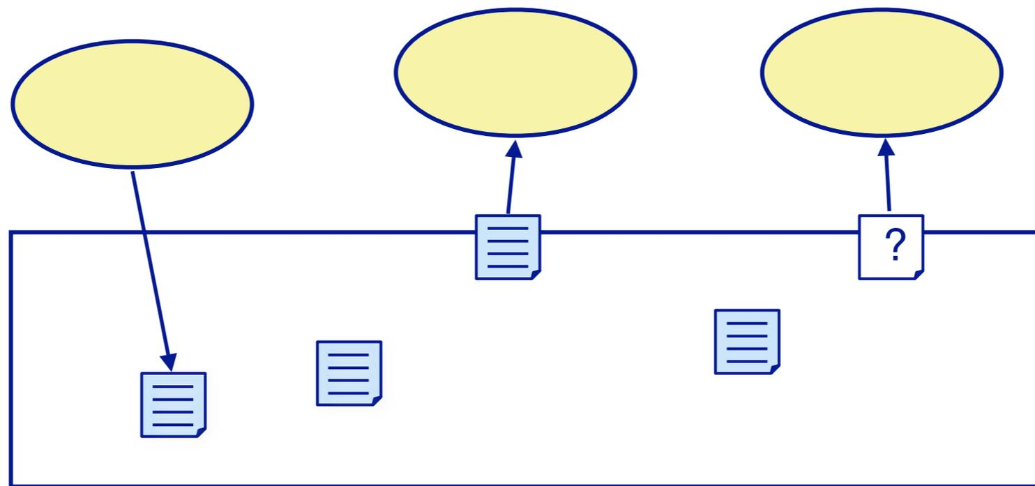
Agents do not exchange messages directly, but post messages to the blackboard, and retrieve messages either by reading from a specific location (i.e., a channel), or by posing a query (i.e., a pattern to match).
