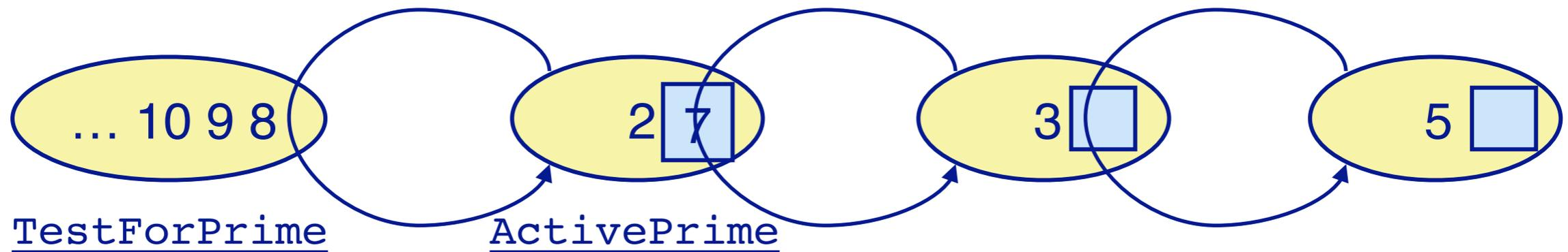
The first ActivePrime holds the seed value 2, gets values from a TestForPrime, and creates new ActivePrime instances whenever it detects a prime value.
