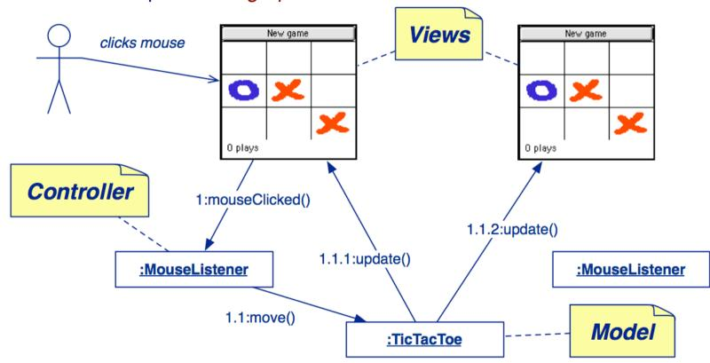
The MVC paradigm separates an application from its GUI so that multiple views can be dynamically connected and updated.
