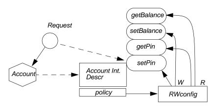
**Figure 6** Configuration of Synchronization policy for accounts: In this example a readers writers policy. The readers writers policy is configured by identifying the set of readers (in this case "getPin", "getBalance") and the set of writers ("setBalance", "setPin")
