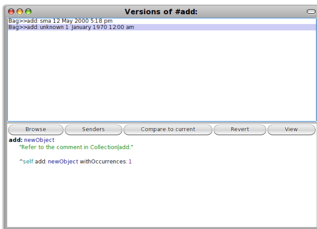
Figure 8: A click on the button labeled “Versions (Git)” shows all the versions of the method #add of class Bag that were found in the GIT repository.
