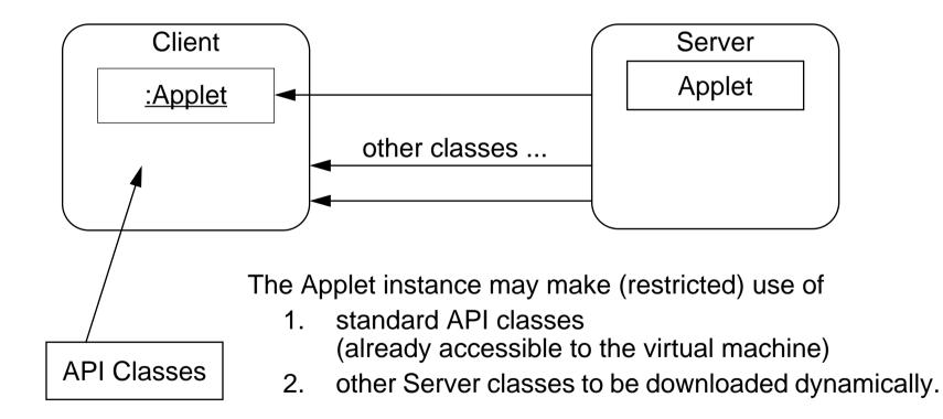
java.applet.Applet extends java.awt.Panel and can be used to construct a UI ...
