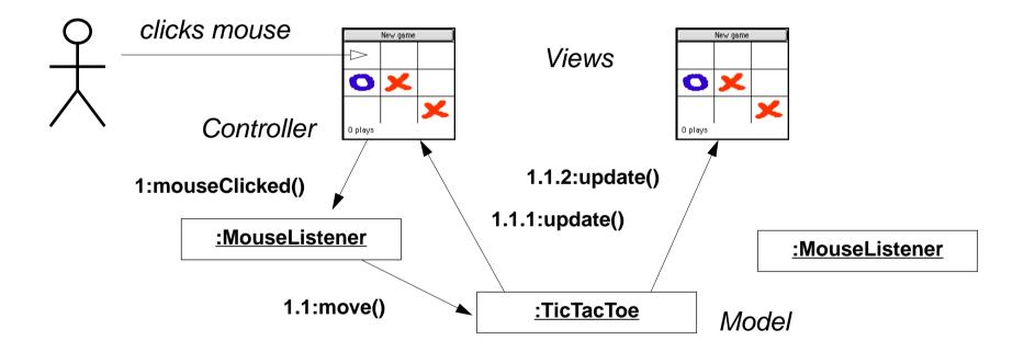
The MVC paradigm separates an application from its GUI so that multiple views can be dynamically connected and updated.
