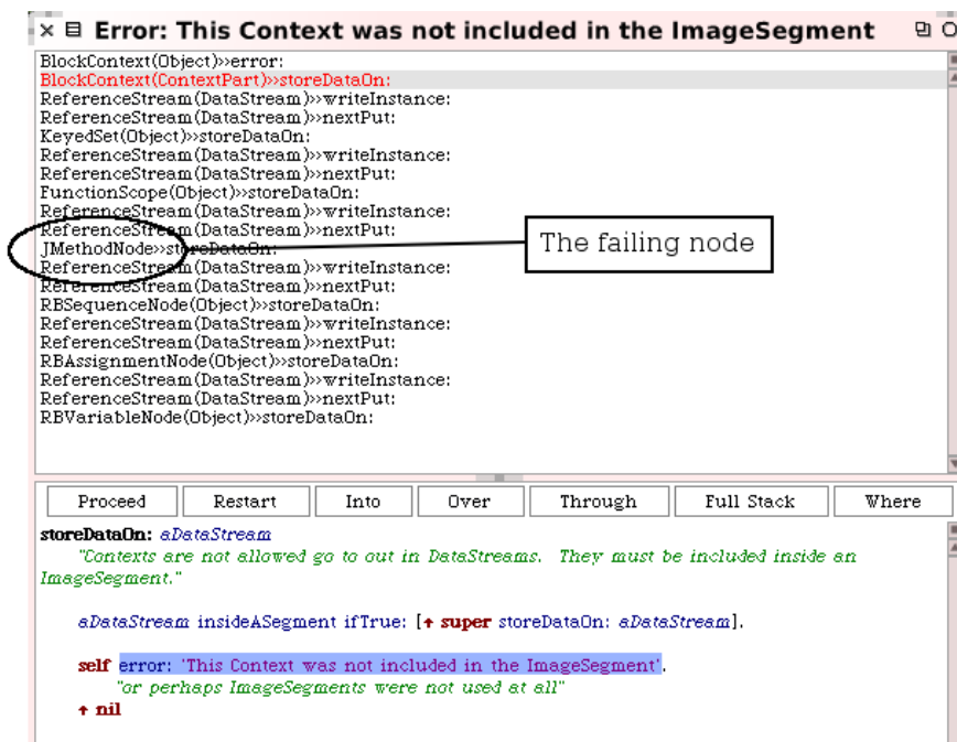
Figure 4.2: The error in the Squeak debugger
