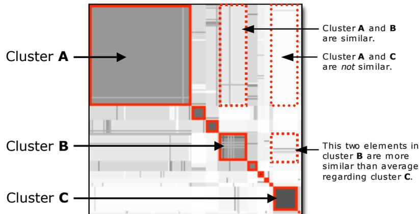
Figure 4.4: A sample *Correlation Matrix*: Cluster *A* and *B* are similar, cluster *C* is very cohesive, two elements in *B* are related to *C*.
