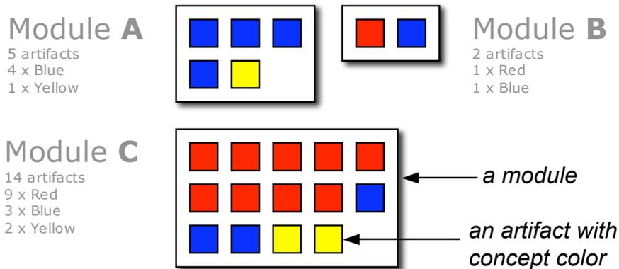
Figure 5.1: The *Distribution Map* shows how semantic concepts are distributed over the structural modularization of a system. Boxes denote modules and software artifacts, colors refer to concepts.
