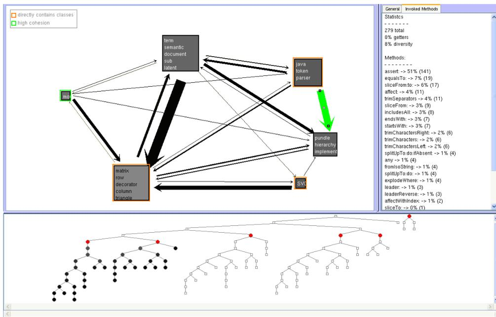
Figure 7.2: Hapax and Softwareaut. On the left: the semantic clusters as boxes with arrows illustrating the number of invocations between them. On the right: the labels for the selected cluster. On the bottom: the dendrogram, a tree view of the clustering.
