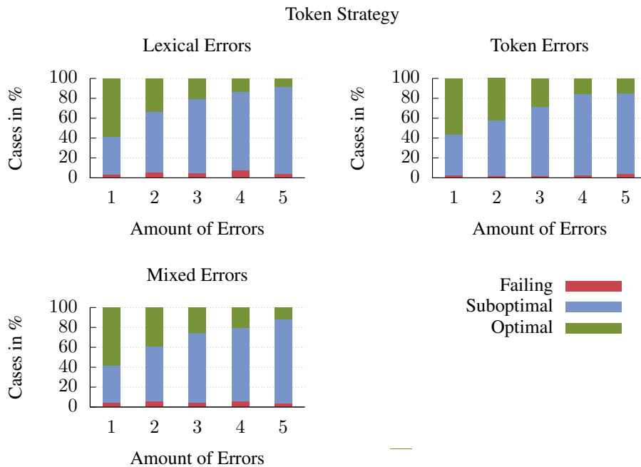
Figure 5.2: Results of the token strategy in presence of lexical, token or mixed errors. The token strategy has a low failure rate in the given setup but also tends to introduce suboptimal results.
