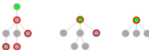
Figure 2.3: Each node of the tree is a package and each leaf is a class. The tree shows the hierarchy of the packages. For each node, red outline shows incoming dependencies while circle fill with green show outgoing dependencies. This figure represents variants of a typical pattern called Iceberg. Iceberg is when the rest of the system knows only the root package
