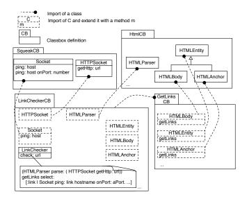
Figure 2: The dead-link checker modularized with classboxes.
