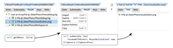
Figure 9: Performing a navigation scenario involving objects that are not directly linked through instance variables: extract the context menu of a list morph, run an action from the menu and verify the result. The first pane shows the tree morph, the second the context menu and the last the current value from the clipboard. At each step code is used to navigate to the next object.
