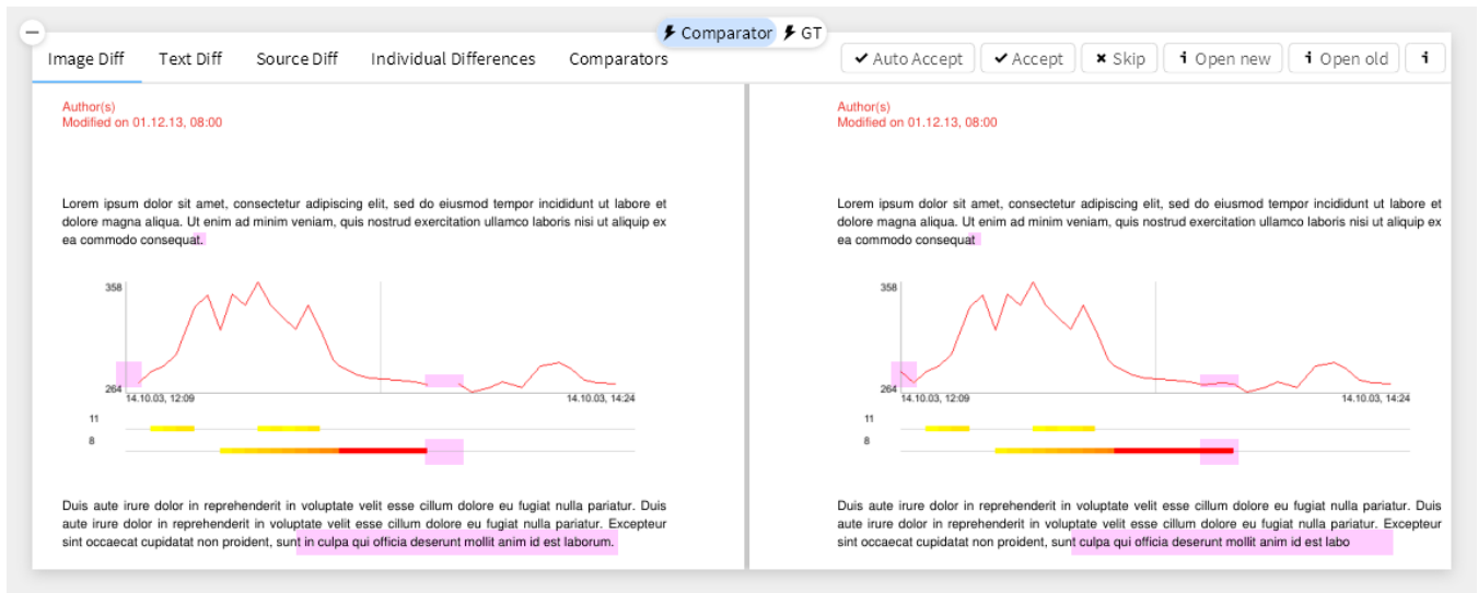
Figure 16. A view showing visual differences between two PDF documents (differences are highlighted in magenta).
