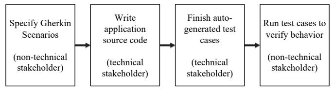
Fig. 1: Typical BDD process
