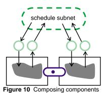
Data ports may be connected to represent data *flow*, or to represent the fact that a port of a composite component is exported from one of its constituent components. For the Petri net procedures, there is no distinction—in both cases, the connected ports represent the *same* shared variable and are therefore modelled by the same, coalesced data place.
