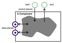
The *behaviour* of the component is a subnet that has read and write access to its data ports. The nature of these subnets depends on the kind of component.
