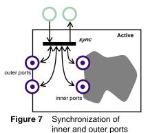
The *outer* ports are never exposed to concurrent accesses, because they are only accessible from the transitions of the outer control net, which contains only a single token.
