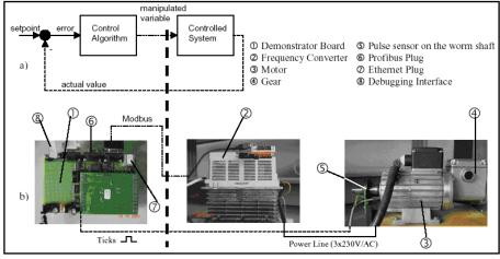
Figure 2 Pecos demonstrator field device
