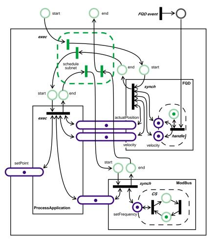
Figure 11 Petri net model of control loop example
