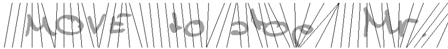
Fig. 1. The input is a line of handwritten text as black-white image. The vertical lines show the output of the algorithm, i.e. the local slant detected by the algorithm.
