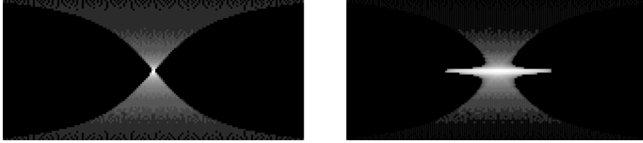
Fig. 7. Illustrates the slant map propagation technique: On the left the butterfly shape of a raw hotspot; on the right the propagated hotspot.
