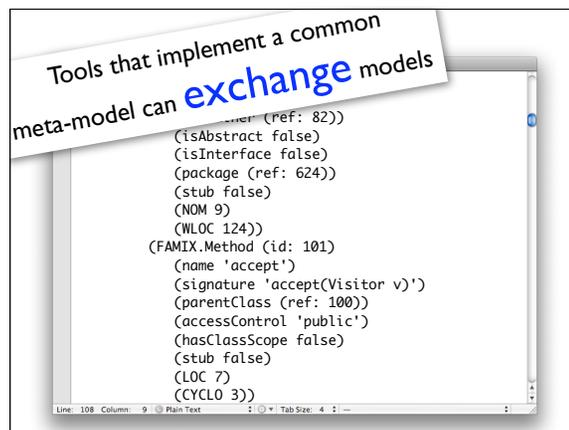
Two tools that share the same meta-model can exchange models that comply with these meta-models by using an exchange format. In this example, we see an MSE file format.
