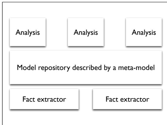
The basic architecture of an analysis tool. Fact extractors extract data from the subject systems. This data is then stored in models that are described by meta-models. Analyses are specified based on the meta-model.
