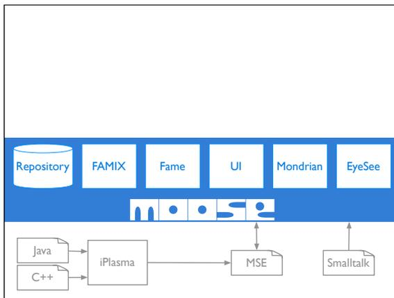
iPlasma is one external tool that can parse Java and C++ systems and exports models complying to FAMIX in an MSE format. These MSE files can then be imported into Moose.
