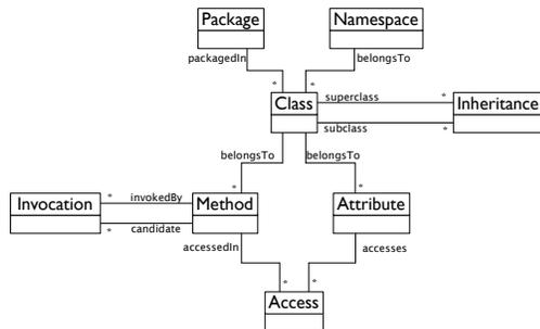
The picture shows FAMIX 2.1. Note how there are no arrows, which means that the relationships can be navigated in both directions. For example, an attribute can know about the accessing methods by going through all accesses that point to him and collecting the methods that initiate those accesses.
