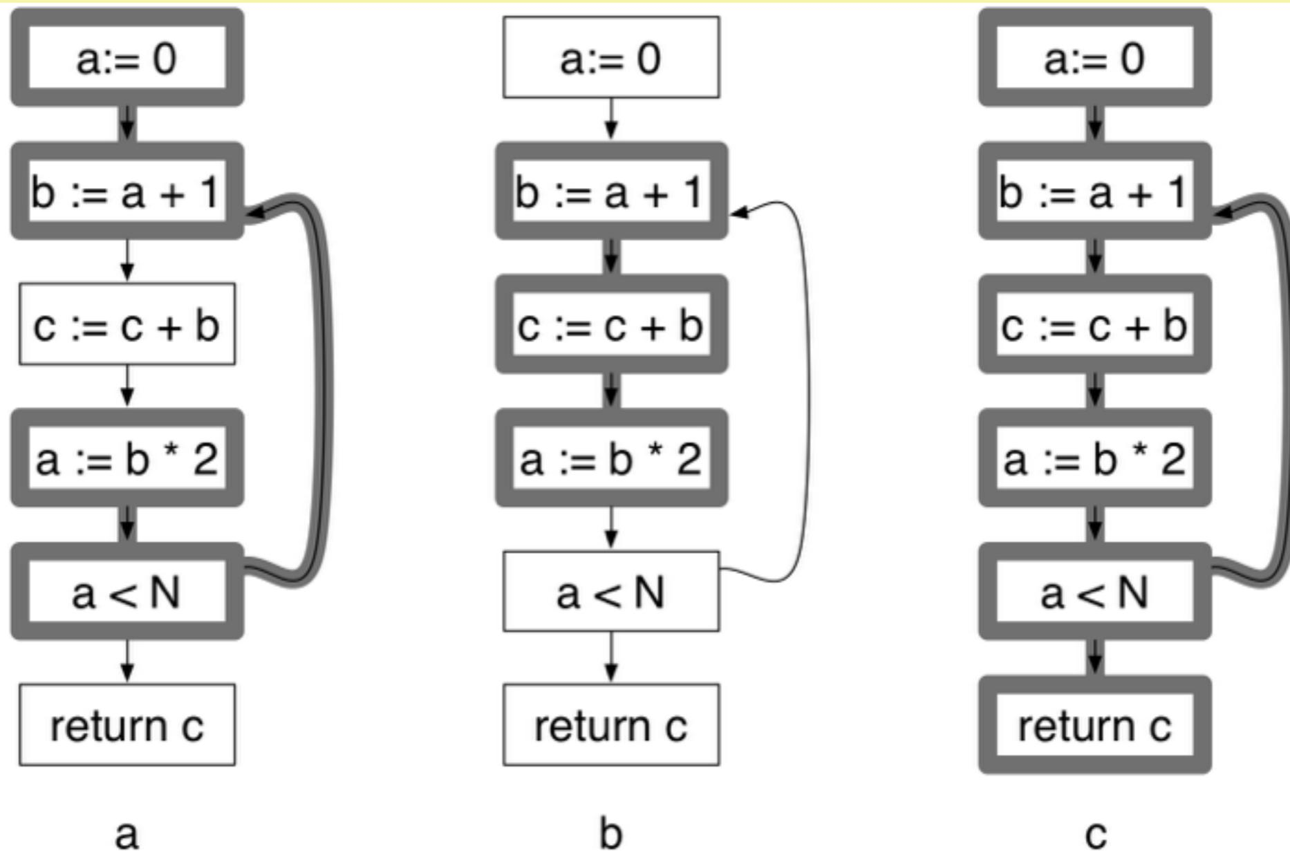
*a and b are never live at the same time, so two registers suffice to hold a, b and c*
