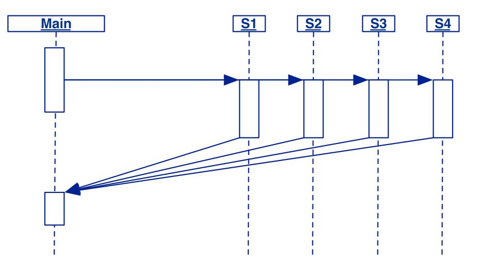
The "cobegin/coend" statement was introduced by Dijkstra as more structured alternative to fork and join. Its main disadvantage is that only a fixed number of processes or threads can be created.
