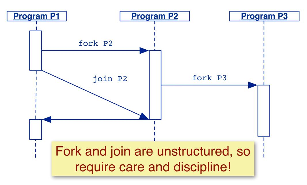
The "fork and join" mechanism is the most common way to create processes or threads. For example, it is used by both the Unix O/S to create (heavyweight) processes and by Java to create (lightweight) threads.
