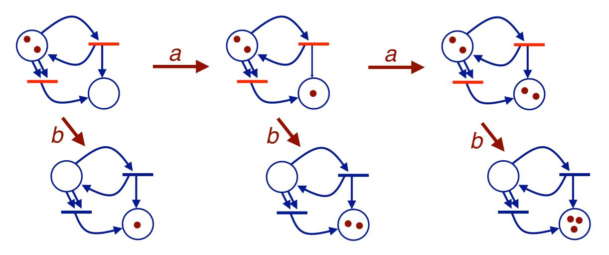
This diagram shows how the net of the previous slide can lead to various possible sequences of transitions being fired. Note that the "*language*" of a Petri net consists of the set of possible firing sequences. In this case, the language can be expressed as a regular expression.
