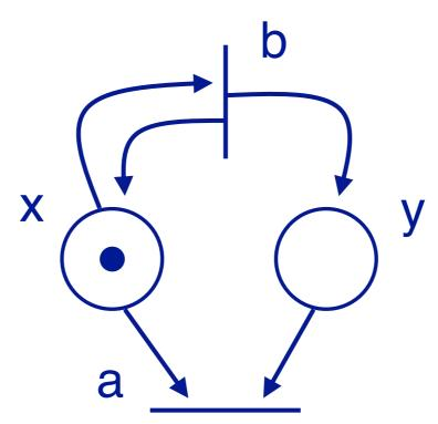
If a and b are implemented by independent processes, and x and y by shared resources, this net can deadlock even though b is enabled if a (incorrectly) grabs x and waits for y.
