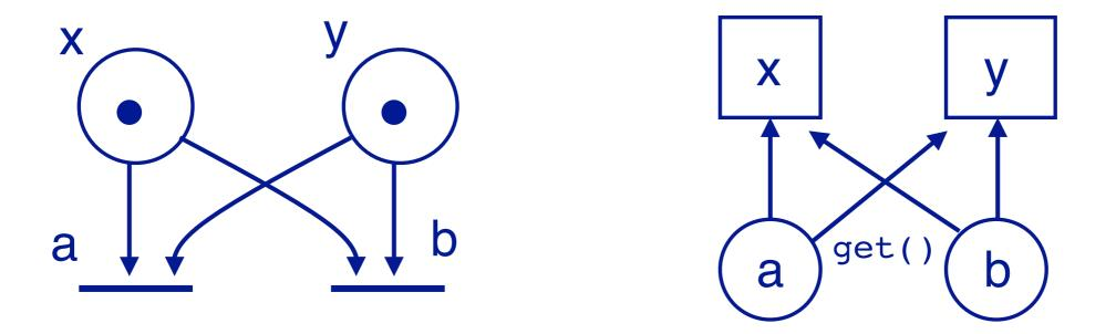
Transitions can be implemented as *thread-per-message gateways* so the same transition can be fired more than once if enough tokens are available. The idea is that the availability of a token in a place will trigger a new thread in transitions that input that place.
