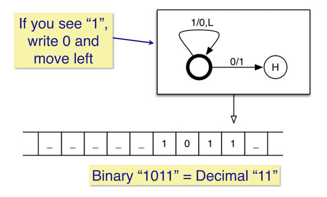
A Turing machine consists of a Finite State Automaton (FSA) and a tape with a finite number of non-blank symbols. The FSA is always positioned at location on the tape. Each execution step consists of:
