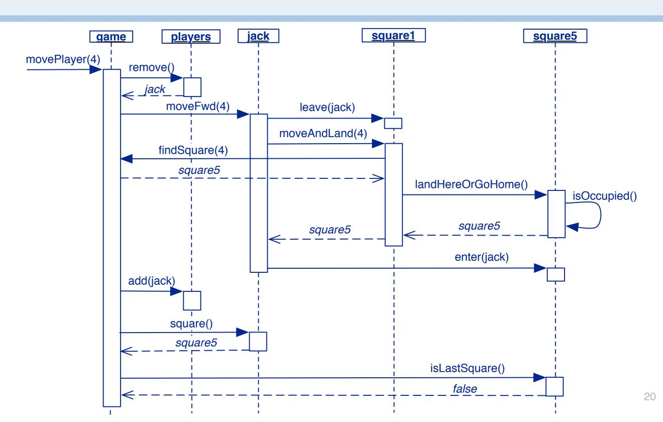
This is a UML sequence diagram tracing a concrete scenario of the first move of a game:
