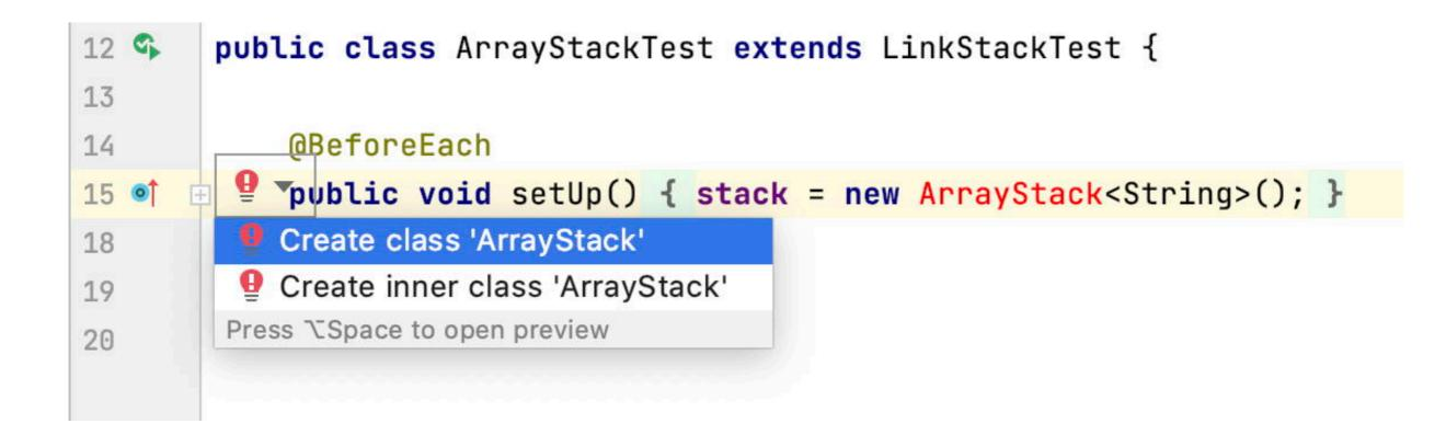
IDEs like IntelliJ recognize that the class you want to test does not exist yet, and can propose to generate it for you as a "quick fix".
