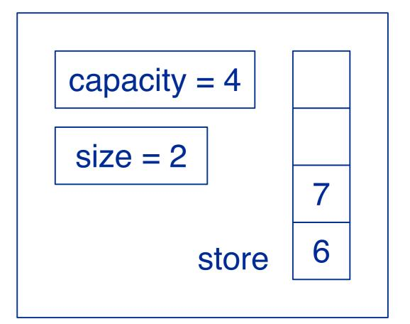
Note that it is not obvious which approach is better. The LinkStack grows and shrinks with every push or pop. An ArrayStack only grows when it runs out of space. A push or pop is very cheap with an ArrayStack, unless it runs out of space, when an expensive copy operation must be performed. It is also not clear what size the initial capacity of an ArrayStack should be, nor how much it should "grow" when a larger store is needed.
