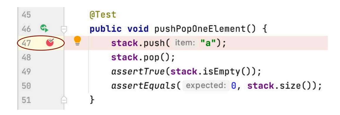
Set a breakpoint within the failing test method (double-click in the margin of the code browser to the left of the line number so a dot representing the breakpoint appears). Then execute "Debug As" JUnit test (i.e., rather than "Run As").
