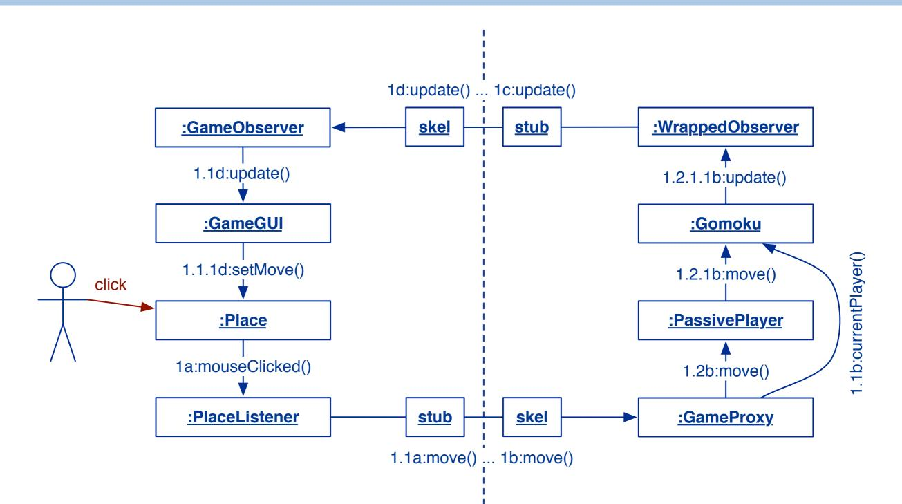
Now we can clearly benefit from our separation of GUI and game logic. The GUI runs on client machines and the game logic runs on the server. Although translating the game to work with RMI is not trivial, the impact on our existing design is quite limited. We only have to introduce remote objects at the points where we cross the boundary between the client and the server.
