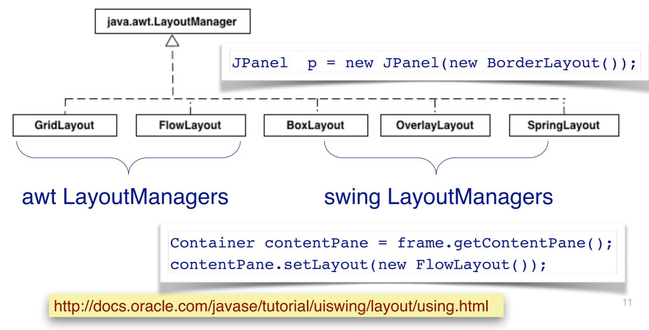
A layout manager is an object that implements the layout manager interface and determines the size and position of the components. Although the components can provide size and alignment hints, a container has the final say on the size and position of the components.
