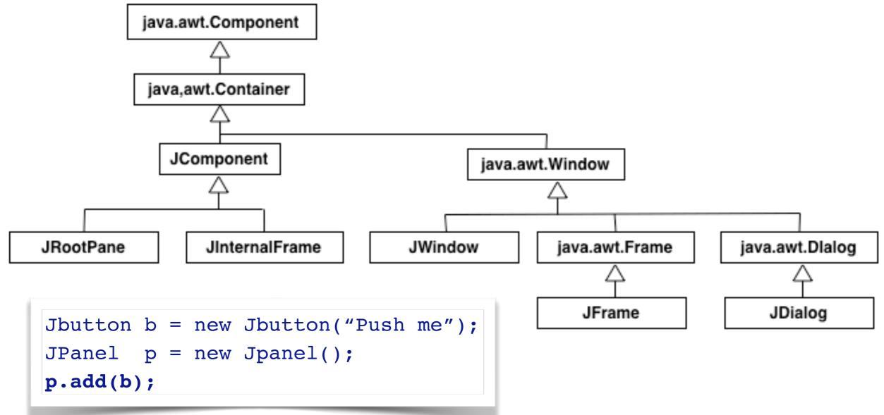
In order to create a GUI, components must be arranged inside a container. A container is a component that can contain other components. Main application windows, dialog boxes are commonly used containers.
