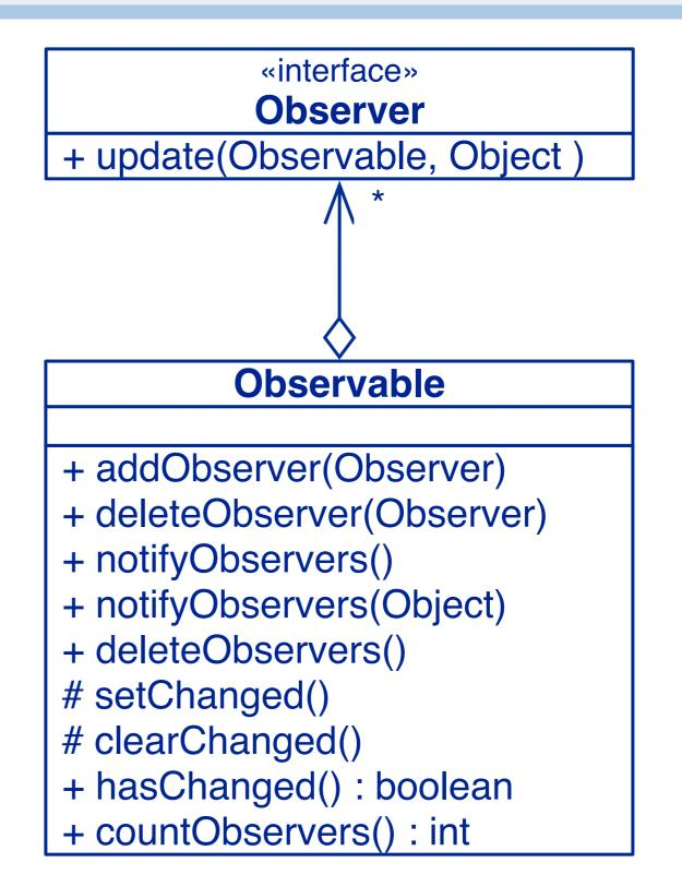
In Java, Observer is an interface providing an update() method. Any object can be an observer by implementing this simple interface.
