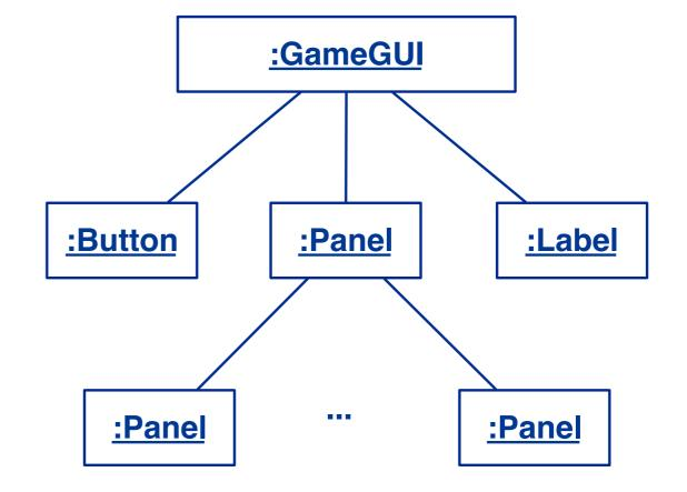
The central Panel itself contains a grid of squares (Panels) and uses a GridLayout.
