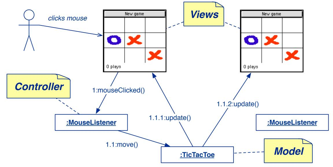
The MVC paradigm separates an application from its GUI so that multiple views can be dynamically connected and updated.
