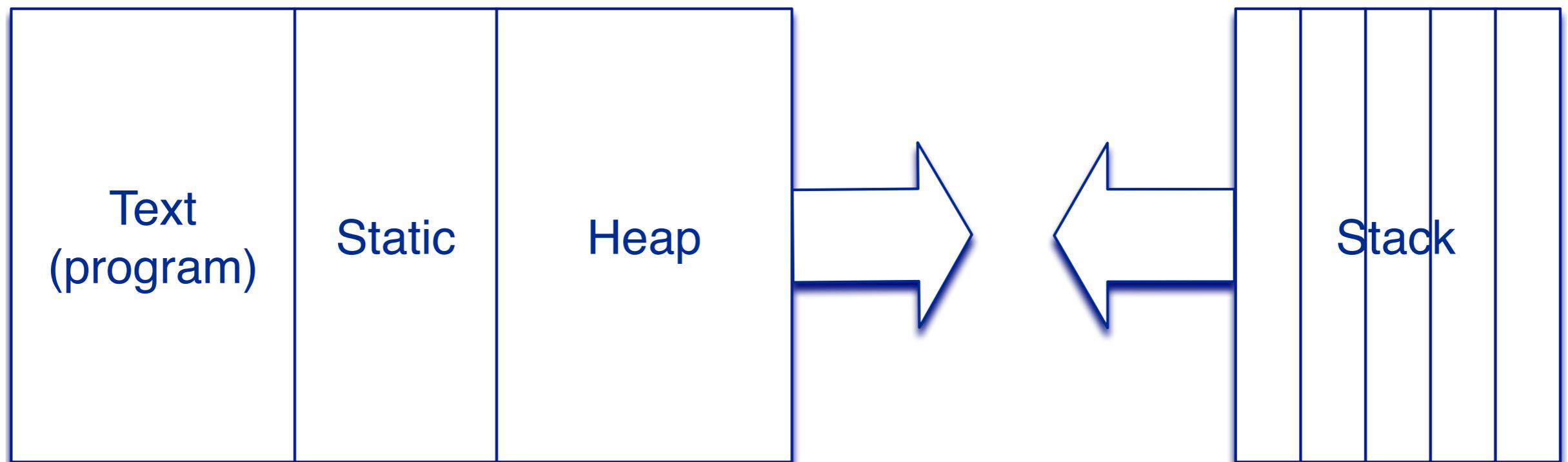
In a classical 32-bit architecture, a 32-bit C or C++ pointer can address up to 4GB of memory. Modern architectures support 64 bit pointers, which overcome the 4GB limitation.
