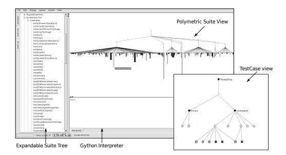
Fig. 1. TESTQ visualizing the test suite's topology.
