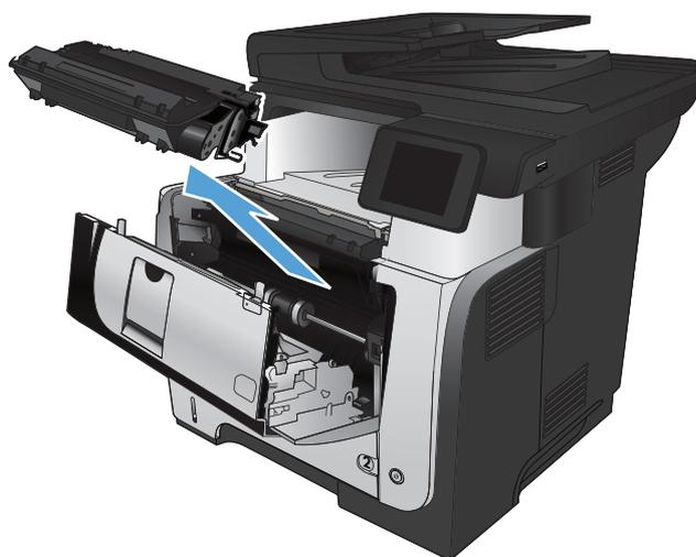
4. Lift the jam-access covers and remove any jammed paper.
