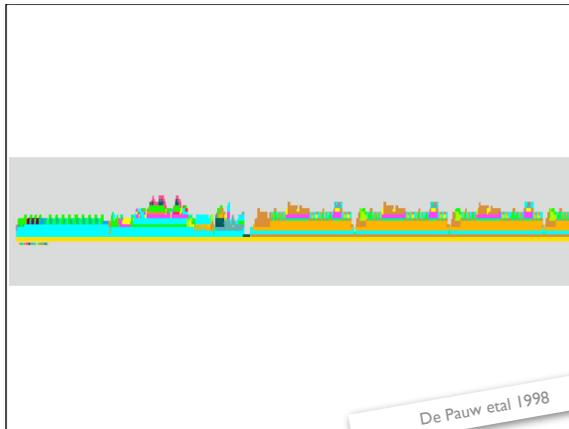
This picture shows a compressed view an execution trace. The orange line at the bottom represents the root of the tree, and the dots from on top represent the leaves of the tree. The colors denote various activation types and reveal repeating patterns.
