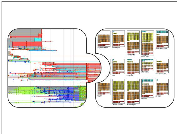
Here we show an example of how we can combine two analyses (namely, ownership map and feature views) to obtain identify how developers work on features.
