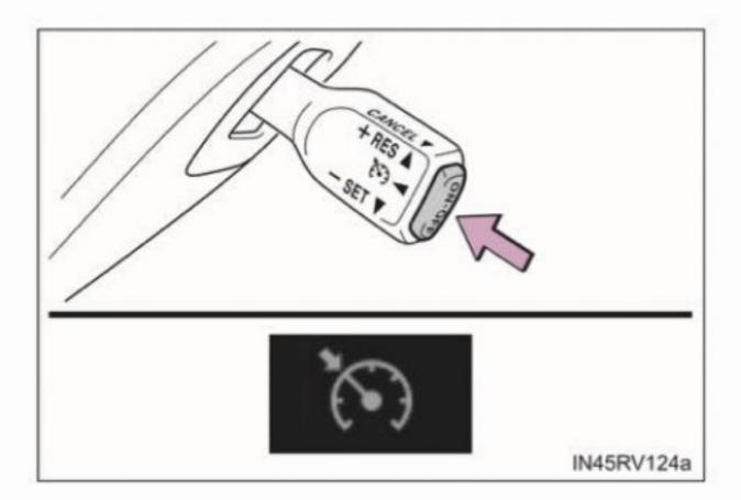
Press the "ON-OFF" button to activate the cruise control. Press the button again to deactivate the cruise control.
