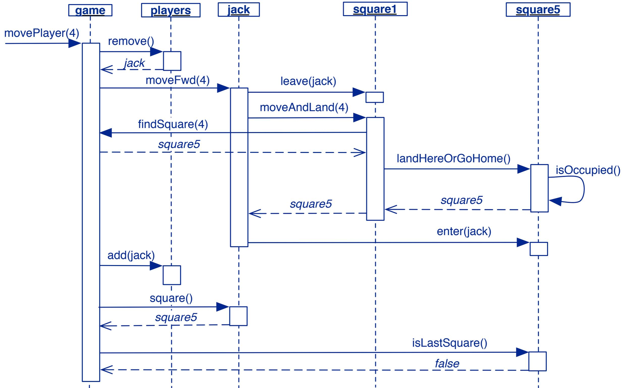
This is a UML sequence diagram tracing a concrete scenario of the first move of a game:
